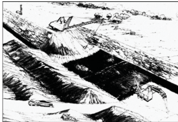
»»» Strip mining with dragline (on overburden) and rope shovel (below, loading coal)
