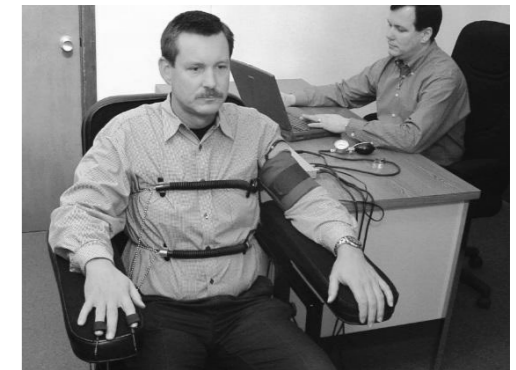
A modern lie detector, combining sensors for breathing rate across the chest, blood pressure on the arm and galvanic skin response on the fingers.
